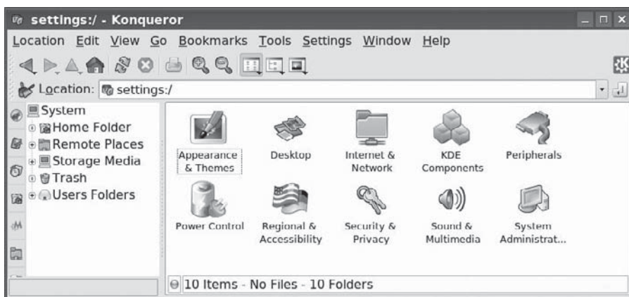
FIGURE 7-7 System settings access (Control Center) from the file manager.
